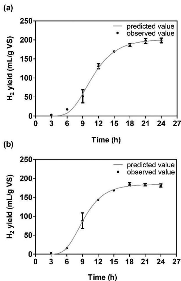
**Fig. 4** – Biohydrogen production kinetics of lipid-extracted algal residues of *Dunaliella primolecta* (a) and *D. tertiolecta* (b) by *Thermococcus eurythermalis* A501. Kinetic analysis conditions were as follows: microalgal residue concentration 2.5 g/L, initial volume ratio of gas to liquid 2:1.
