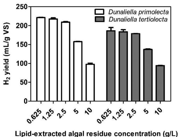
Fig. 2 – Effects of algal residue concentrations on SHY of *Thermococcus eurythermalis* A501.
