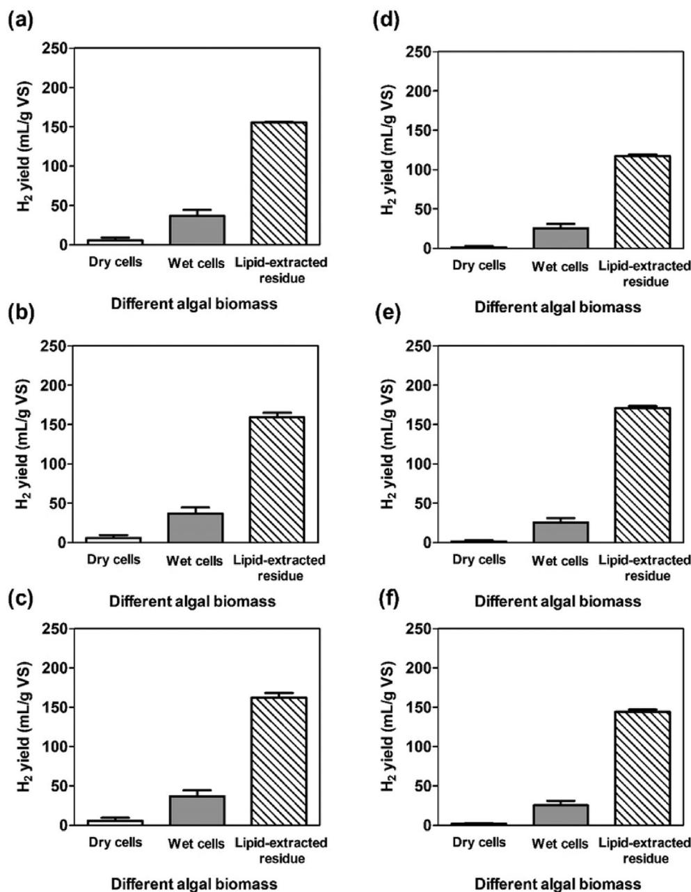
**Fig. 1** – SHYs from different algal biomass of *Dunaliella primolecta* (a, b, c) and *D. tertiolecta* (d, e, f) by *Thermococcus eurythermalis* A501. a, d: Different algal biomass under the same initial biomass concentration; b, e: different algal biomass under the same initial carbohydrate concentration; c, f: different algal biomass under the same initial protein concentration.
