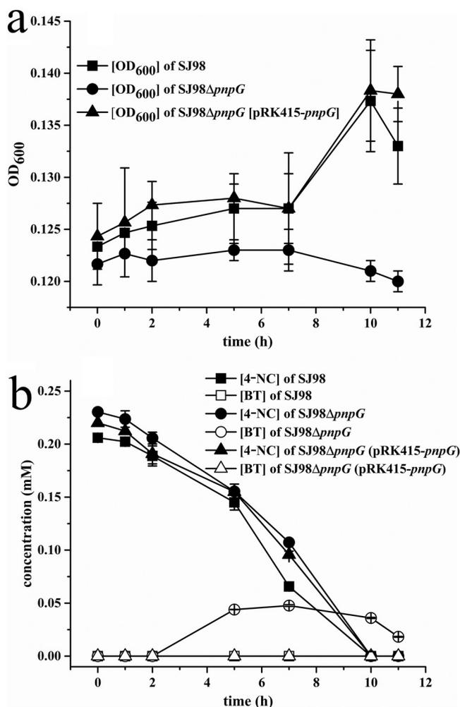
**FIG 3** Time course assay of 4-NC degradation and the growth of *Burkholderia* sp. strain SJ98 and its derivatives. Strains were grown in MM with 0.2mM 4-NC as the sole carbon source at 30°C. (a) Growth curves of strain SJ98 and its derivatives on 4-NC. (b) The consumption of 4-NC and the accumulation of BT were quantified by HPLC. The symbols indicate the means for three replicates, and error bars indicate standard deviations of the means ( $n = 3$ ).
