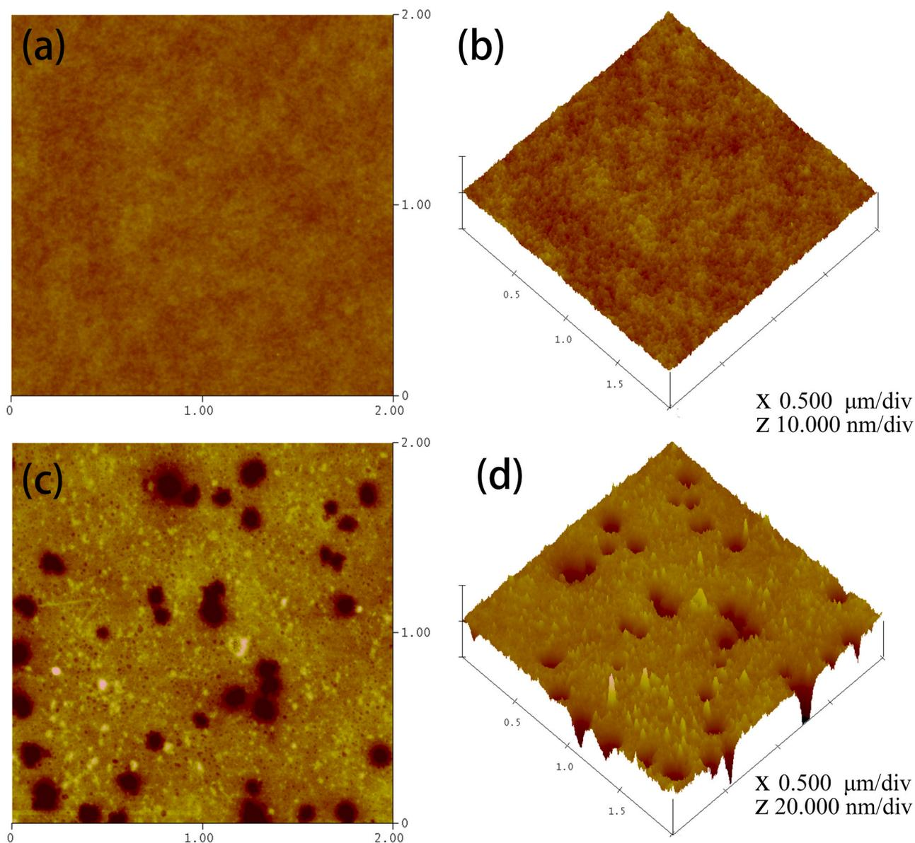
**Fig. 1.** Two dimensional (2D) and three dimensional (3D) atomic force microscope (AFM) images of the physical surface topography: (a) 2D and (b) 3D images of the control sample; (c) 2D and (d) 3D images of the PC films treated by strain NyZ600 for 30 days.
