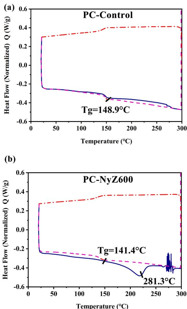
Fig. 4. Differential scanning calorimetry (DSC) curves of heating and cooling cycles of sample. (a) control; (b) treated sample (PC films incubated with strain NyZ600 for 30 days). The solid line represents the first heating process; the dash-dotted line represents the first cooling process; the dashed line represents the second heating process.
