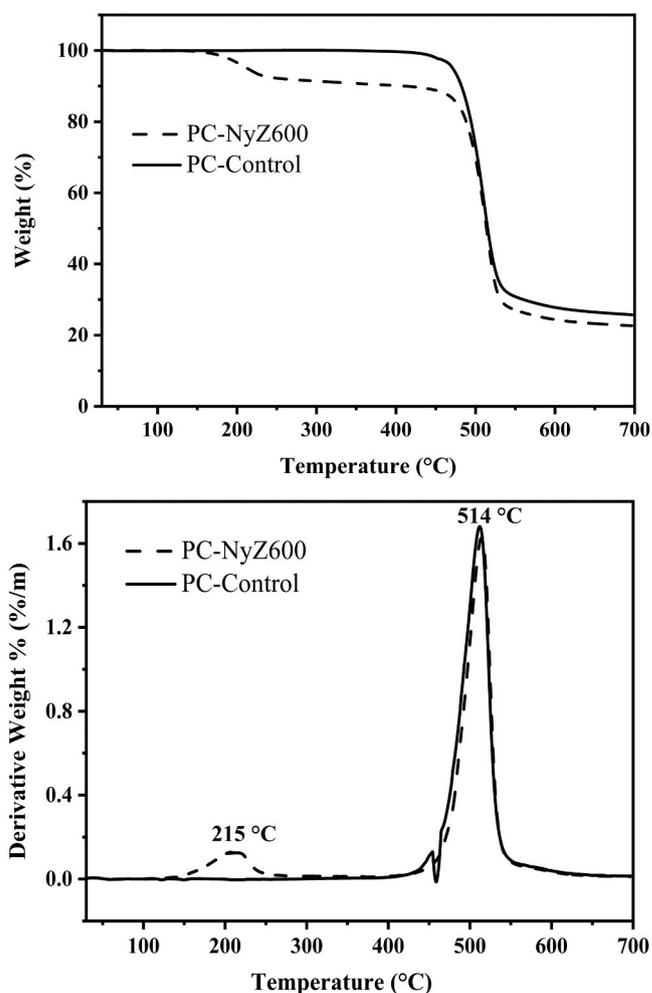
Fig. 5. Thermogravimetric analysis (TGA) (upper panel) and differential thermogravimetric (DTG) (low panel) curves of the control and the PC films treated by strain NyZ600 for 30 days.
