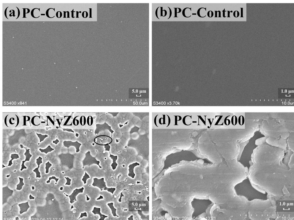
Fig. 2. Scanning electron microscopy (SEM) images of the control sample (a and b) and PC film degradation by strain NyZ600 for 30 days (c and d). An ellipse indicates the presence of bacterial cells (c).
