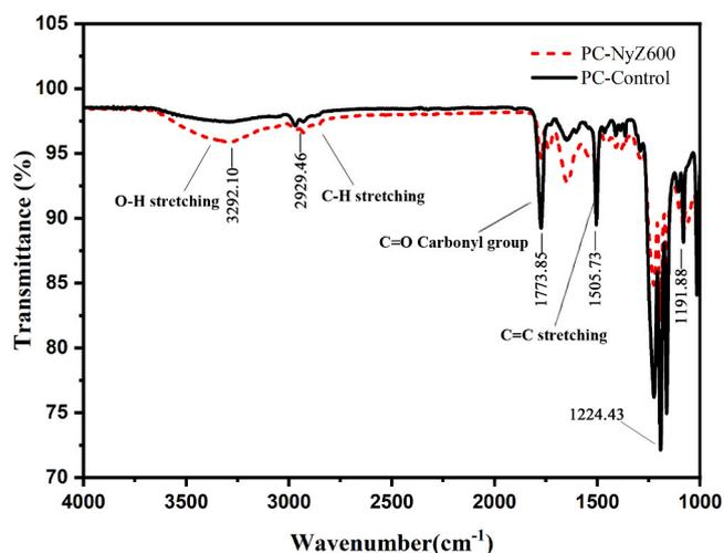
**Fig. 7.** Fourier transform infrared (FTIR) spectra of control sample (solid line) and PC plastic film treated with strain NyZ600 after 30 days (dashed line).
