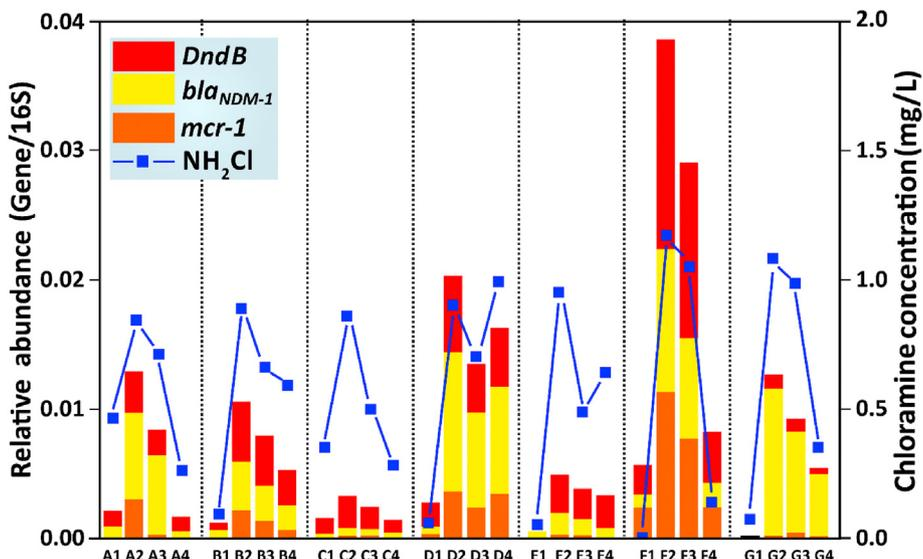
**Fig. 2.** Relative abundance of *mcr-1*, *bla<sub>NDM-1</sub>*, *dndB*, and chloramine concentration in different waterworks. A–G: seven different water treatment plants; 1: waterworks influent; 2: waterworks effluent; 3: primary water supply system; and 4: secondary water supply system. The vertical lines in the figure are shown to distinguish between each water treatment plant.
